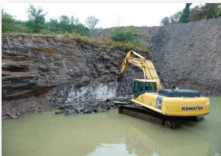
Mechanical extraction of stone from the quarry
